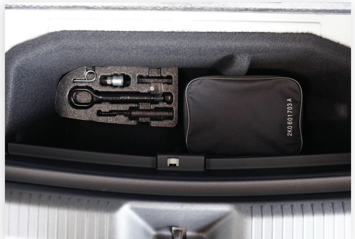
Roadside kit under load floor in trunk
