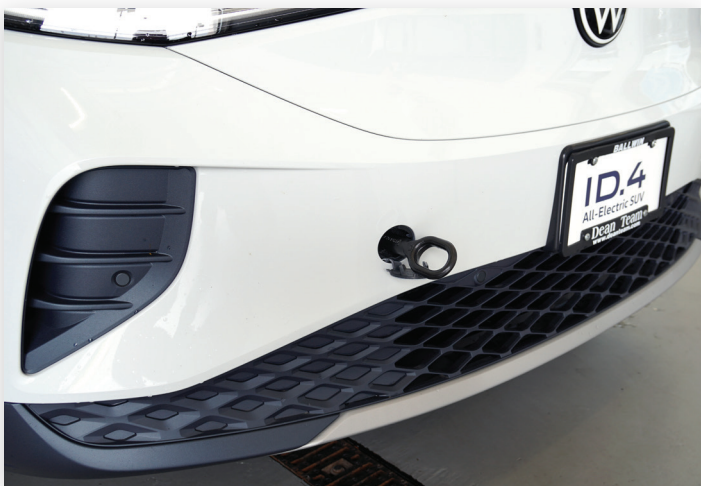
Tow eyelet is left-hand thread
